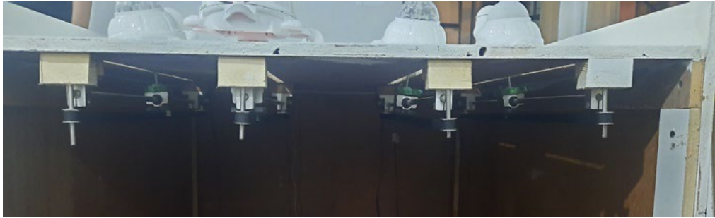
Figure 5 Row of stepper motors driving synchronized rotational movement of turtle toys in Age of Bibitulit.
